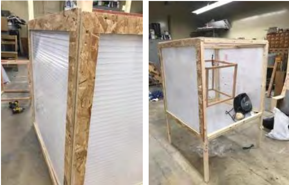
Figure 2a: Cubical box with Aerogel glazing
