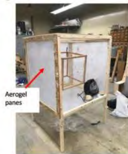
Figure 1: View of cubical scaled room
