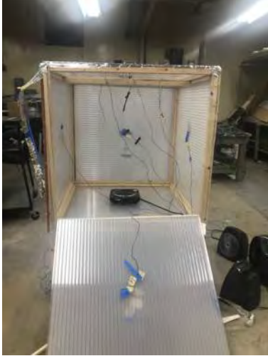
Figure 2c: Cubical box with sensors attached
